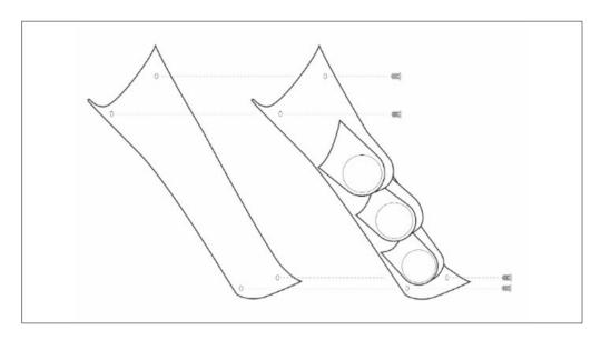
Note: This gauge pod mounts directly overtop of your vehicle's factory A-pillar and is not a complete replacement.
