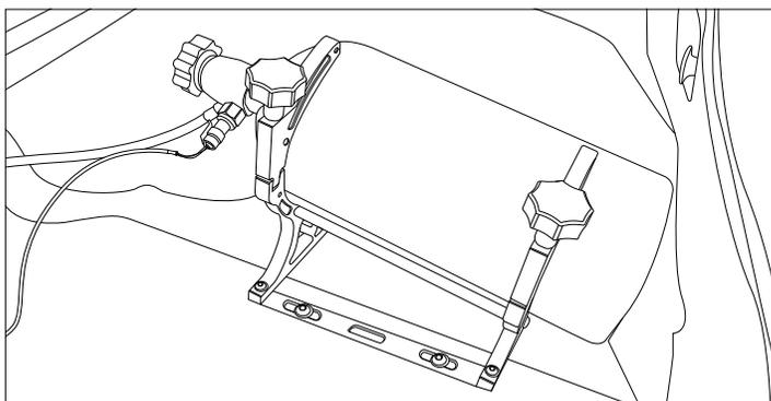
There are a few different ways to connect a Nitrous Pressure Gauge to your vehicle. In most cases an adapter is needed to adapt the 1/8-27 NPT Sensor to your system.
