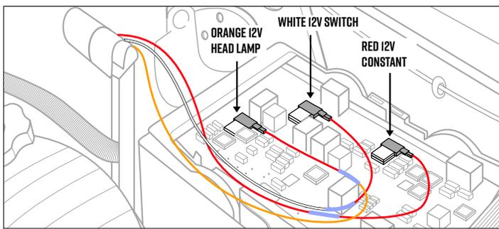
5. Repeat the same step for the **White Wire** of the gauge to locate an Ignition Switched 12-Volt Power Source. This source should not have any power with the key turned off and have 12 volts with the key turned on.
