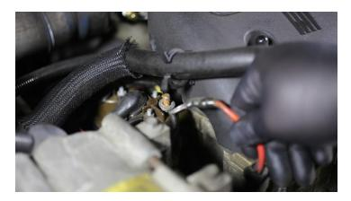
4. Using a 10mm wrench, remove the captured nut and power wire from the stud on the IAH. Once this has been removed, you can then remove the power wire from the IAH.
