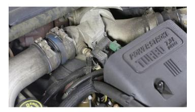
3. There is a power wire that runs from the IAH down to the solenoid. This is the main power wire for the Intake Air Heater Element. Using a 13mm wrench, remove the nut and washer from the solenoid and disconnect the power wire from the solenoid. This power wire is what energizes the heater element.
