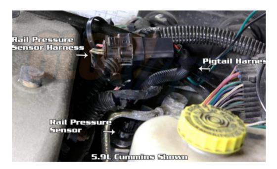
This fuel rail pressure pigtail harness is compatible with the 2003 - 2012 5.9L & 6.7L Cummins and 2002 - 2018 Duramax LB7, LLY, LBZ & LMM diesel engines.
