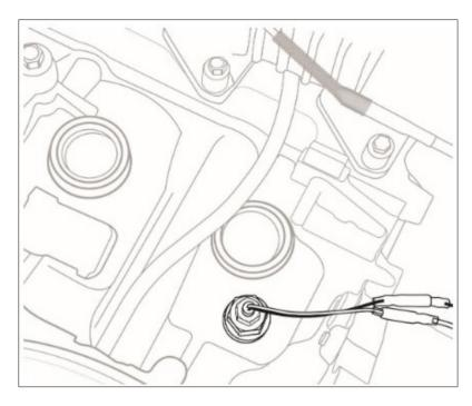
The Ford 6.0 Power Stroke Water Temperature Sensor Adapter allows you to install a temperature sensor into a coolant passage on the driver side of the engine block.
