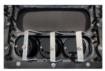
This 3 gauge dash mount will only work with vehicles that are 2WD or have a manual shifter for 4WD. This product WILL NOT work with electronic controlled 4WD.
