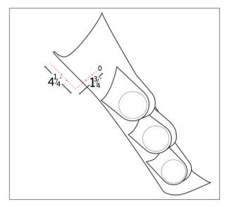
Note: This pillar pod is a complete replacement and will require removal of the factory A-pillar trim.
