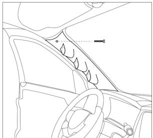
Note: This pillar pod is a complete replacement and will require removal of the factory A-pillar trim. Be sure to store the factory A-pillar trim in a safe location when done.
