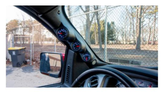
Note: This pillar pod is a complete replacement and will require removal of the factory A-pillar trim. Be sure to store the factory A-pillar trim in a safe location when done.
