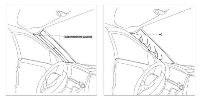
Note: This pillar pod is a complete replacement and will require removal of the factory A-pillar trim if applicable.
