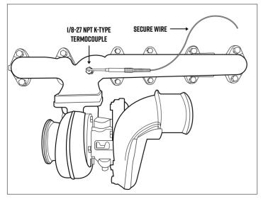
2. Starting with a **1/8" Drill Bit** drill a hole at the marked location stepping up to a size **"R" Drill Bit**. A 1/8-27 NPT Drill and Tap Set can be purchased at MaxTow.com.
