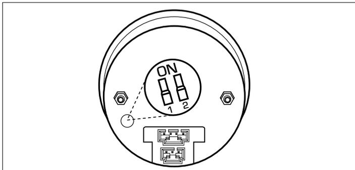
2. Plug the Fuel Rail Pressure Sensor Harness into the back of the gauge.
