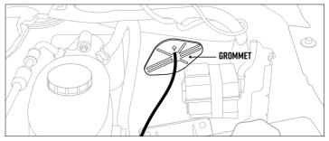
Plug the Intake Temperature Sensor Harness into the back of the Intake Temperature Gauge.
