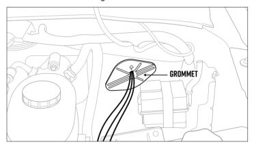
5. Plug the Boost Pressure Sensor Harness into the back of the Boost Gauge.
